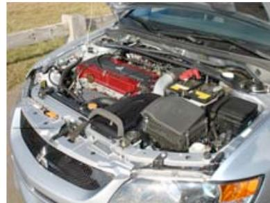
The 2.0 Liter DOH 16 valve 4-cylinder engine produces quite a punch considering its small size. With 286 horsepower, and 289 lb.-ft. of torque the Evo takes off with lightning speed. There are two-scroll turbochargers that not only propel this car to 0-60 in less than six seconds, but also sound like a jet taking off in the process. In
