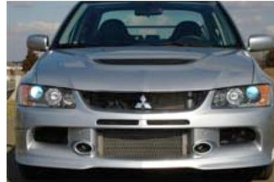
each side of this are oval holes that look like fog lamps but are actually air vents that suck in the much needed cool air to keep the engine at optimal temperature. The front headlights are a one piece unit that has three circular lamps with the main HID unit tinted in a blue color. The headlights are
